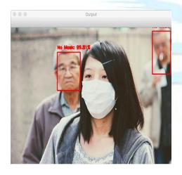
Figure 14: Face Mask Detector Failed to detect person with Mask
